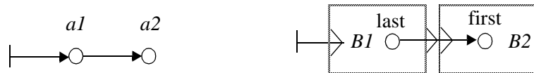
Figure 6.16: Sequence of two actions a1 and a2 , and of two behaviours B1 and B2
